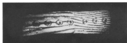
Figure 9 Reconstructed image from hologram of tibia 7. Compression was applied across the fracture site using an AO narrow dynamic compression plate, shown to be less effective by the lower fringe density ratio (FDR) across fracture site.
